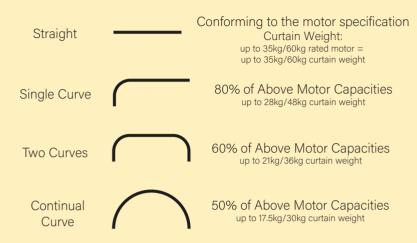
Calculate maximum curtain load in track stacking sections. Do not exceed guidelines.
