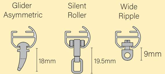
The above dimensions for both 25 mm and 35 mm profiles are the same.
